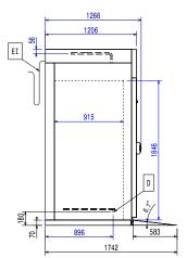
Electrical inlet (power) ΕI RO Refrigerant Outlet
